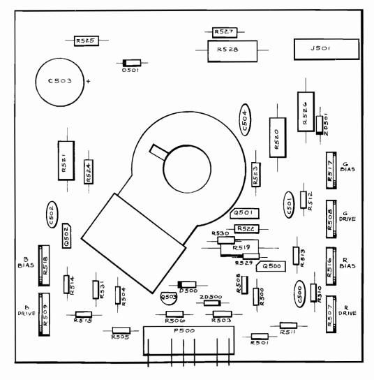
Figure 14 Neck PCB Assembly 99-130479 C
