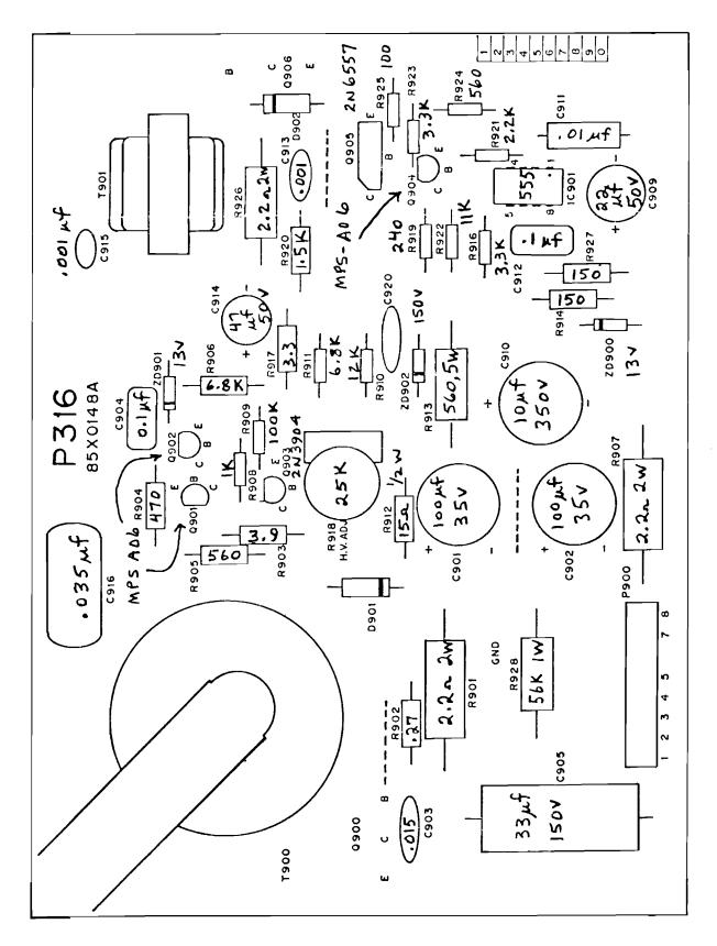
Figure 15 High-Voltage PCB Assembly 99-130490 C
