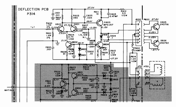
Figure 7 Schematic Diagram of Y Amplifier
