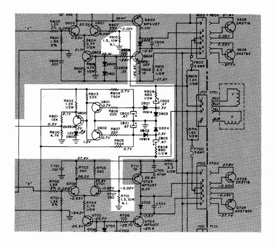
Figure 9 Schematic Diagram of Spot Killer Circuitry
