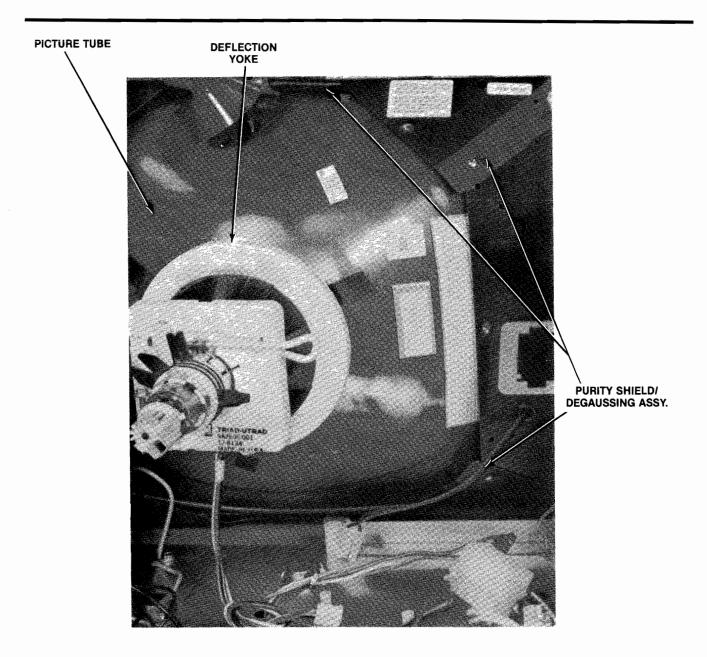
Figure 12 Display Assembly 92-053 C
