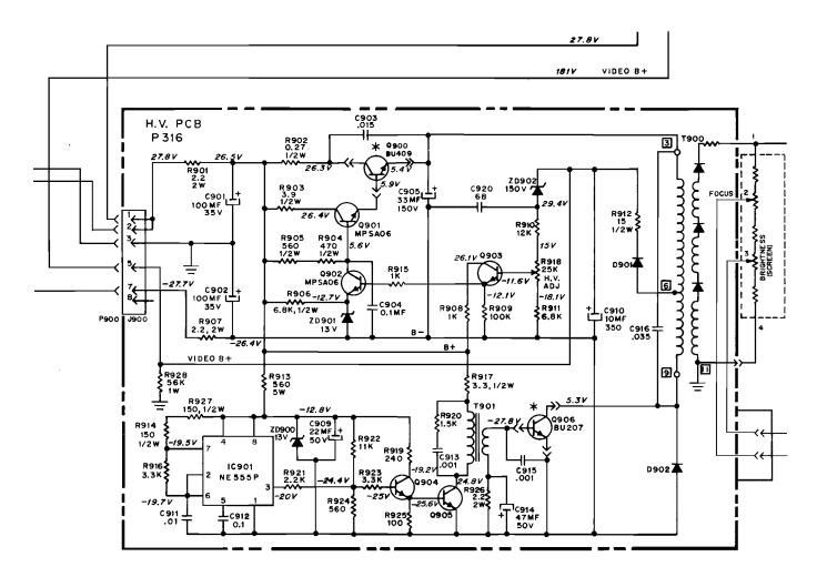
Figure 10 Schematic Diagram of High-Voltage Power Supply
