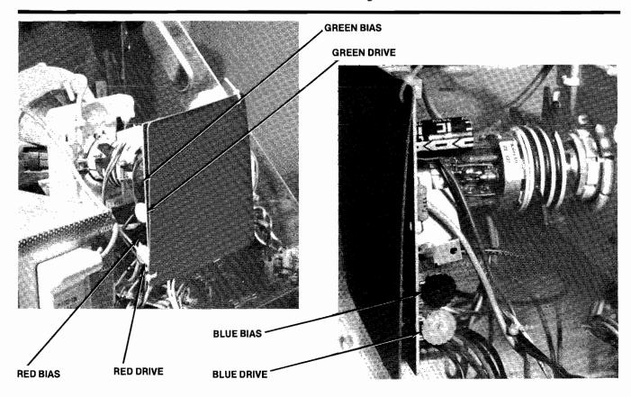
Figure 4 Adjustable Controls on Neck PCB
