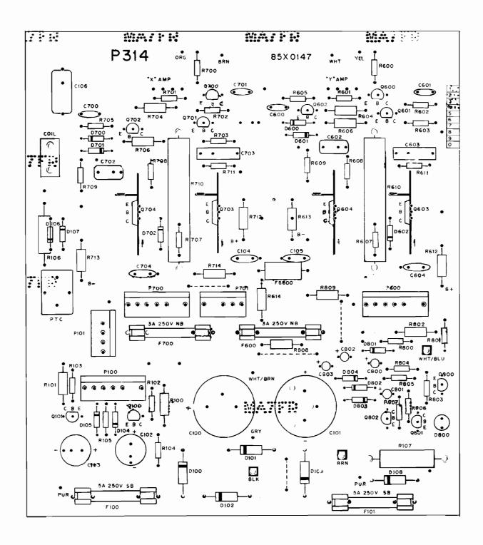
Figure 13 Deflection PCB Assembly 99-130474 C
