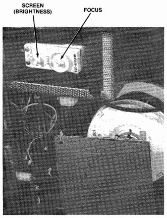
Figure 2 Adjustable Controls on High-Voltage "Cage"
