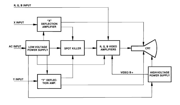
Figure 5 Display Block Diagram
